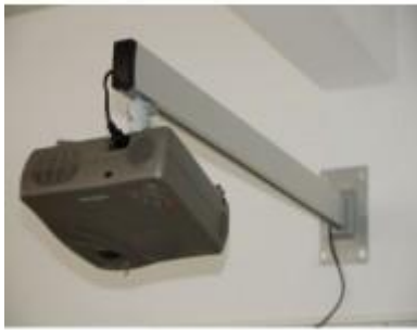
Reflecta Vesta 120 ; length 1250mm; inclinable 30°; max load Projector 15kg
